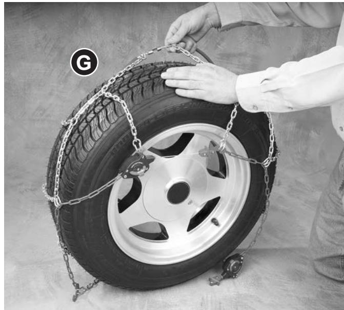
**ENGLISH:** Leave the red lever in the up position and slide the side cable to the back of the tire (G), ensure the chain is centered on the tire.
