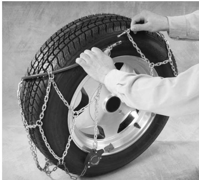
**ENGLISH:** Bring the back side cable forward and disconnect (Refer to Installation instructions, step 2, page 4 ). After use, it is important to wash chains in hot water in order to eliminate salt deposits and prevent rust. Carefully inspect for any worn chains or damaged components. Repair, or remove from service, chains that are worn or chains with damaged components. Dry chains, lubricate with light oil and store in canvas carrying case.
