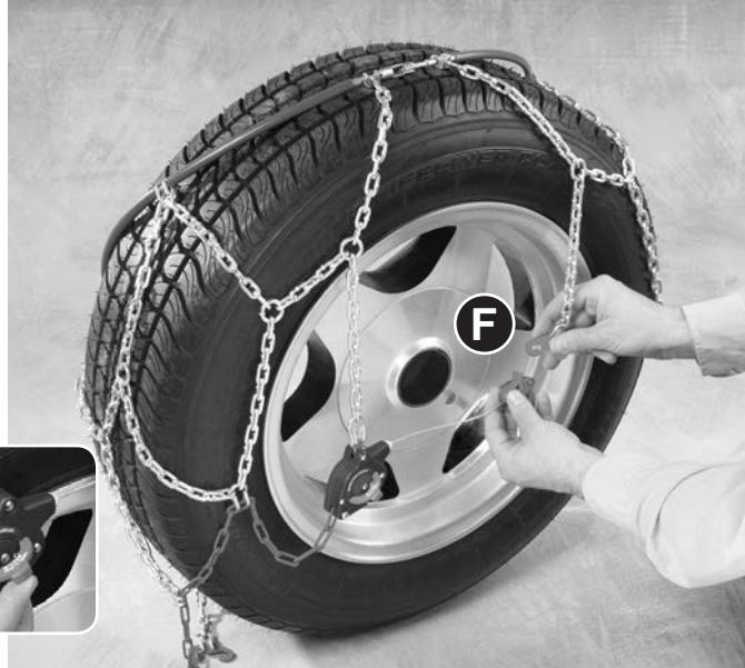
**ENGLISH:** Grasp the top tensioner (E) and flip the red lever up to remove. Pull the red cable end out of the side-chain connector (F). Firmly grasp the red cable end and flip the red lever down to take up the exposed cable.
