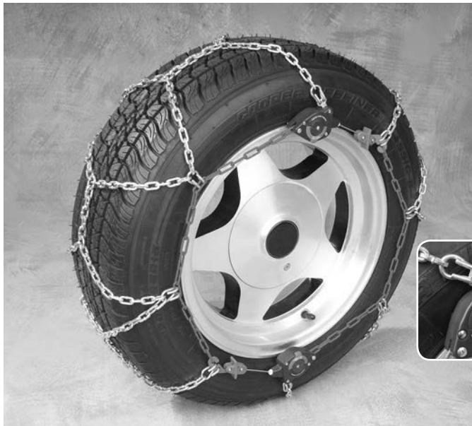
ENGLISH: Flip the red lever down to tighten both the top and bottom tensioners. Your chains will begin to self tighten.
